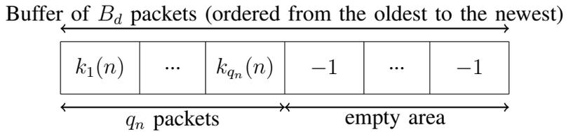
Fig. 1: Buffer configuration at slot  $n$ .
