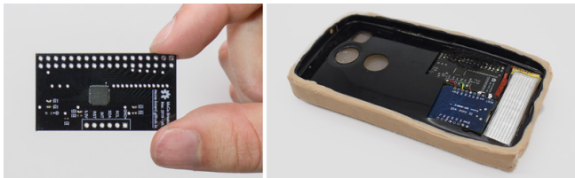
Figure 11. Left. Open Hardware Mutual Capacitance breakout Right. Smartphone case prototype hardware.
