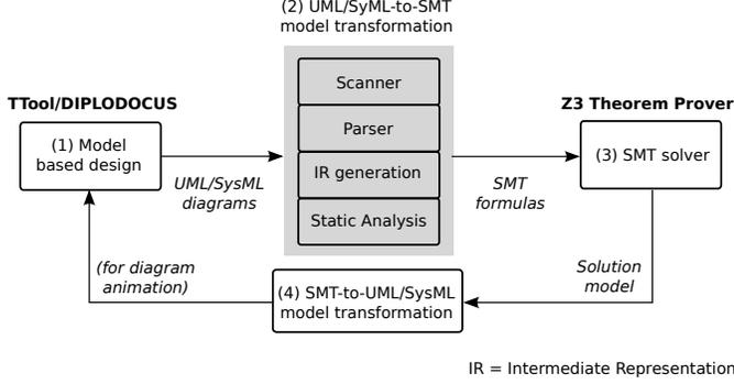
Fig. 1. Overview of the Design Space Exploration workflow.
