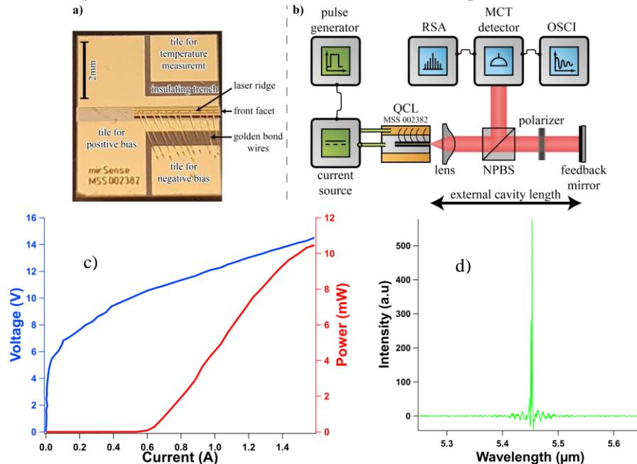
FIG. 1 a) & b) experimental setup split between the analysis path above and the back-reflection path below with a close-up on the QCL chip; c) and d) LIV curves and optical spectrum characteristics of the free-running DFB QCL operating at 77 K under a continuous bias, respectively.
