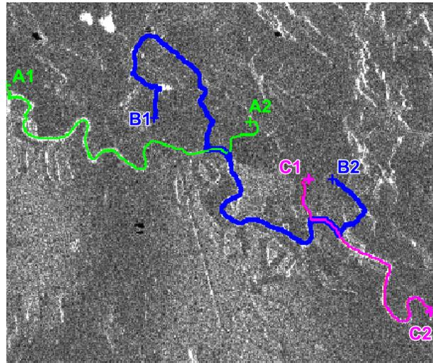
FIGURE 7. Visualization on the same image of the result of the least-cost paths for 3 pairs of nodes :  $A1 \rightarrow A2$  in green,  $B1 \rightarrow B2$  in blue and  $C1 \rightarrow C2$  in magenta. The centerlines have been widened for better visualization. In this example, the a priori nodes have been chosen excessively far from the river to illustrate the robustness of the proposed approach.
