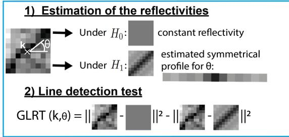
FIGURE 4. General presentation of the linear structures detection performed on the log-transformed images. Example for a patch centered in  $k$  and for dark linear structure detection.
