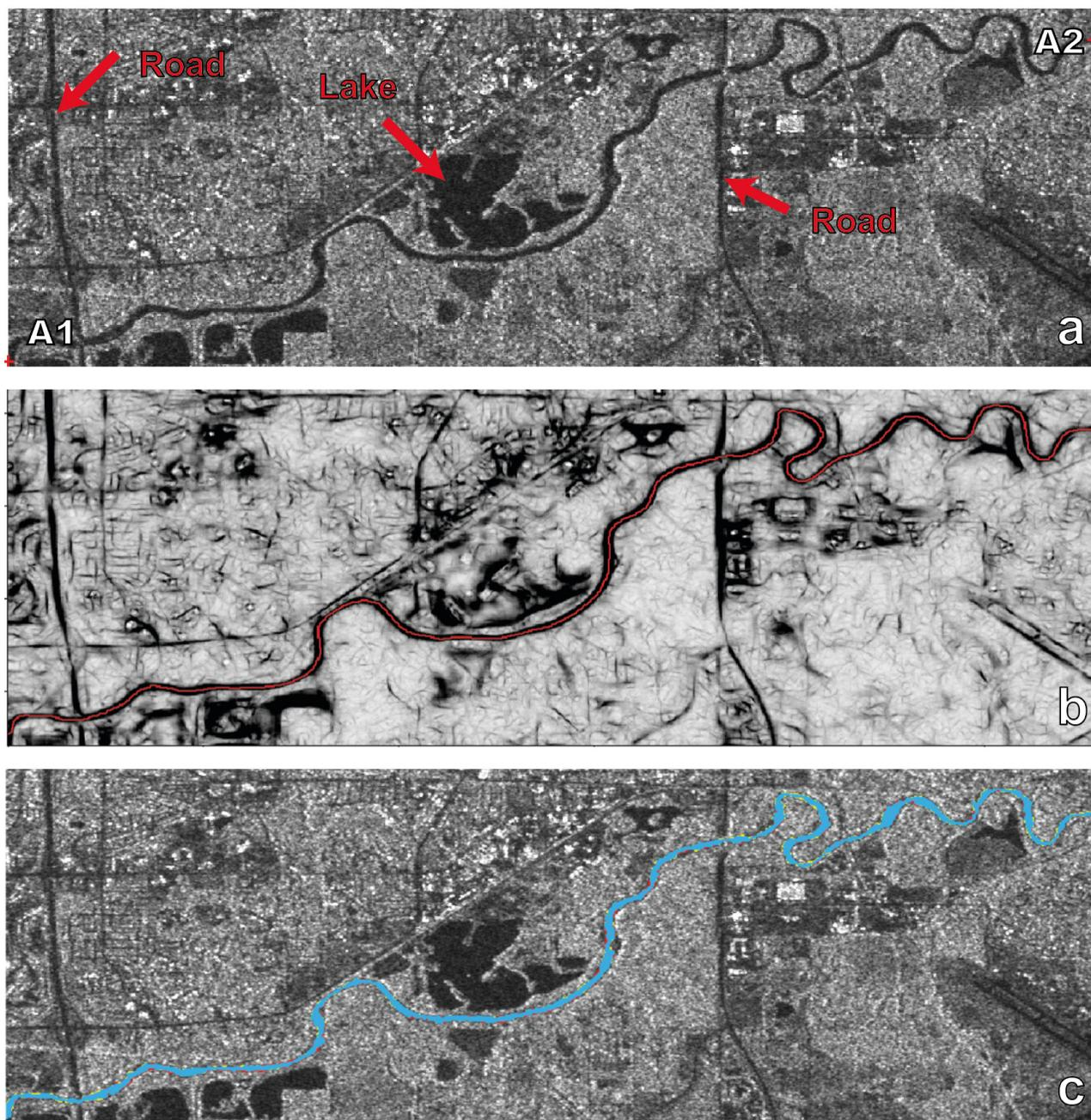
FIGURE 14. Image 1 (Des Moines) : (a) SAR image with annotations, (b) centerline (in red) on the linear features detector and (c) final segmentation. A1 and A2 mark the two nodes used as prior information. The color map of the line detector has been inverted and the centerline has been widened for better visualization. In (c) the true positives are displayed in blue, the false positives in yellow, and the false negatives in red. True negatives are displayed as the actual SAR image pixels.
