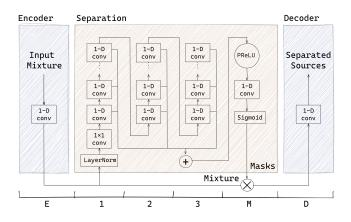
Figure 1: ConvTasnet architecture. Layer names are given below to understand the different fine-tuning strategies.
