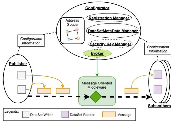
Fig. 3. Prototype of an OPC UA PubSub-C system
