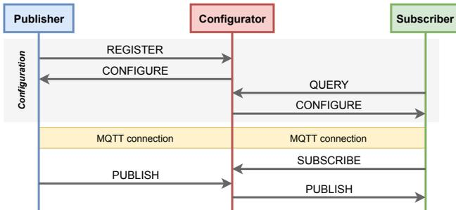
Fig. 5. Exchange between components in the broker-based mode
