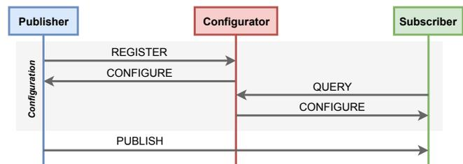
Fig. 4. Exchange between components in the broker-less mode
