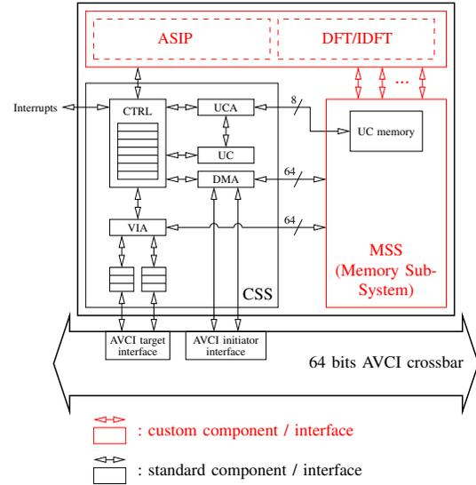
Fig. 3. FEP DSP Unit including the ASIP
