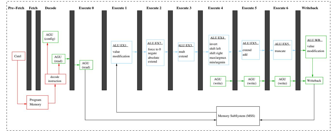
Fig. 4. Pipeline of the ASIP for FEP
