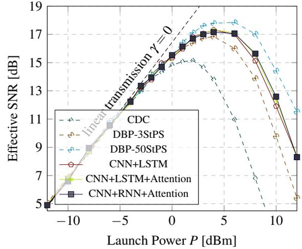
Fig. 3: The effective SNR of the models as a function of the launch power.
