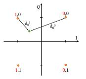
Fig. 5:  $d_0^0$  and  $d_0^1$  representation for bit 0 estimation in a QPSK constellation
