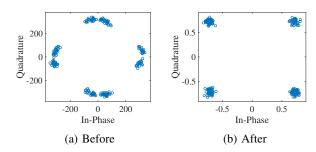
Fig. 4: Samples constellation before and after Channel equalization for PDCCH samples
